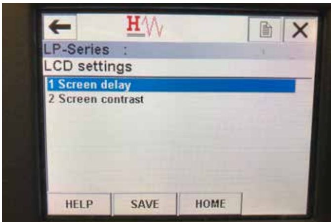
Fig. 31: LCD Settings Menu Screen
