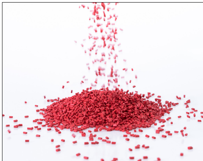
Fig. 2: Plastic granulate for injection molding or extrusion
