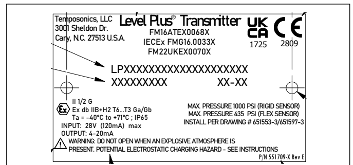
Fig. 59: Flameproof, ATEX/IECEX and UKCA label, HART®, Housing Option D, E, G, H, or L
