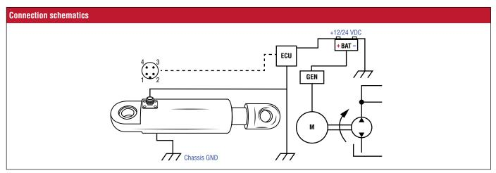
Fig. 6: Connection schematics
