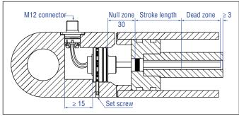
Fig. 7: Example of In-Cylinder assembly
