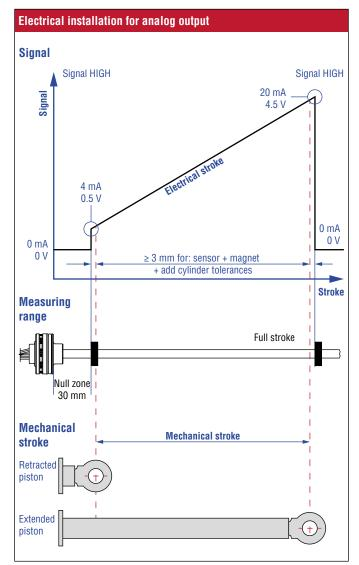
Fig. 10: Electrical installation
