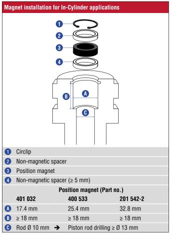
Fig. 11: Dimensions for magnet mounting
