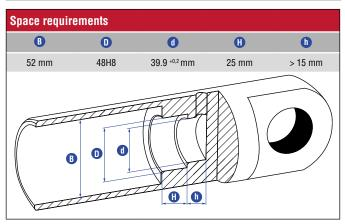
Fig. 8: Space requirements for cylinder
