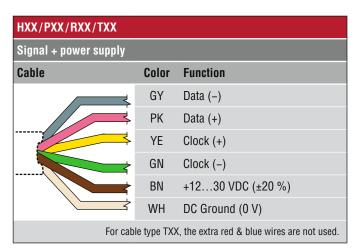
Fig. 4: Connector wiring HXX/PXX/RXX/TXX
