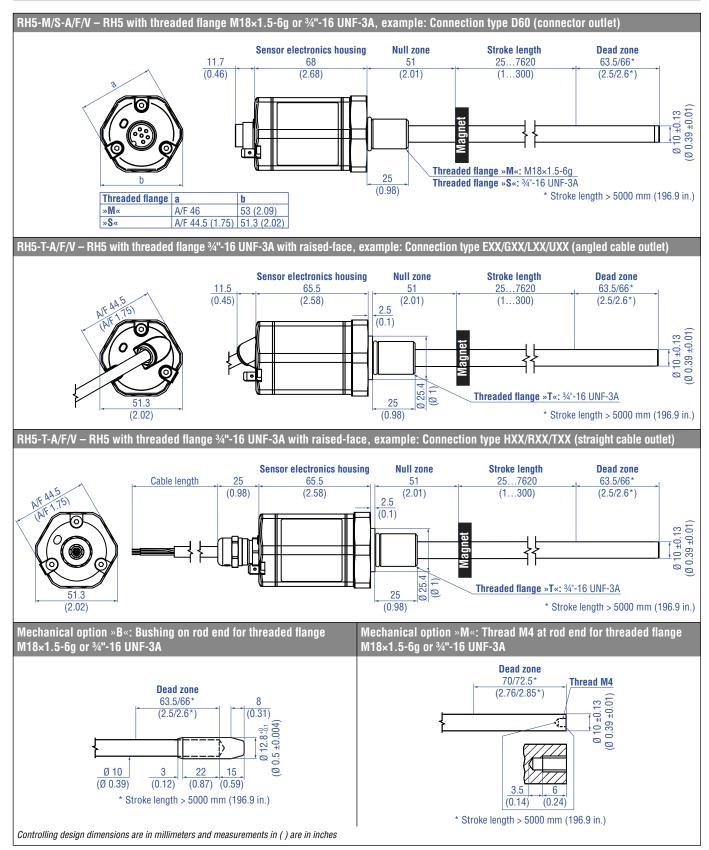
Fig. 6: Temposonics® RH5 with ring magnet, part 1
