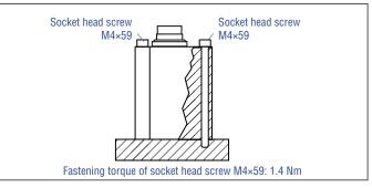
Fig. 22: Mounting with socket head screws M4×59
