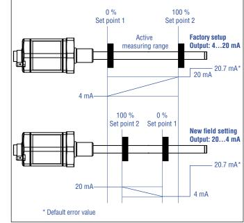
Fig. 83: Reversal of the measuring direction by adjusting the start value (set point 1) and the end value (set point 2)
