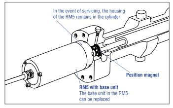
Fig. 14: RM5 sensor in cylinder
