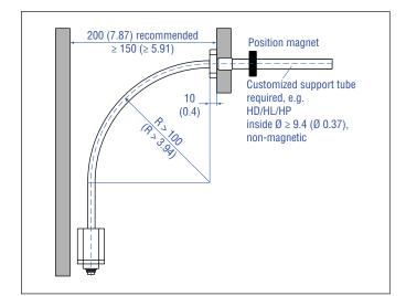
Fig. 20: Clearances for installation and handling
