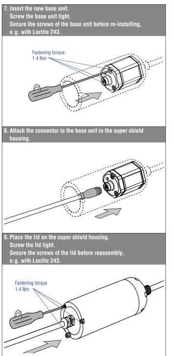
Fig. 70: Replacement of the base unit on model RM5, part 3
