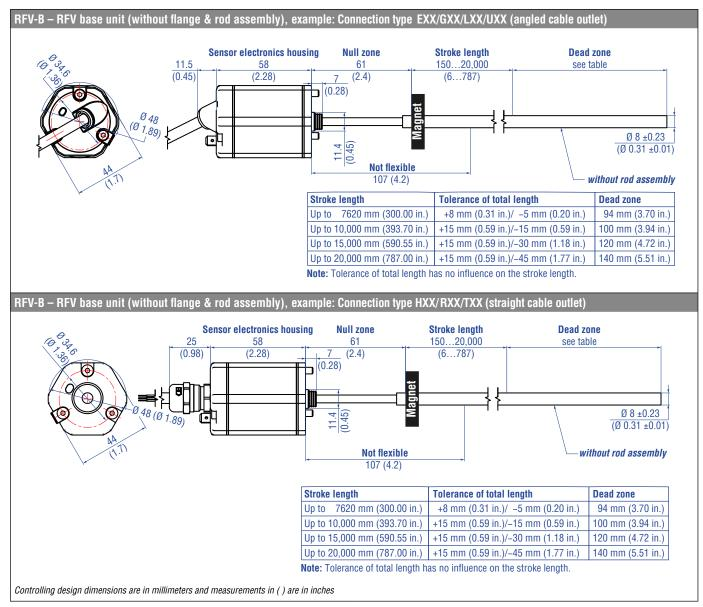
Fig. 29: Temposonics® RFV with ring magnet, part 2
