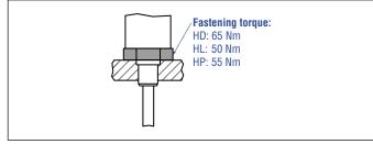
Fig. 24: Mounting example of threaded flange
