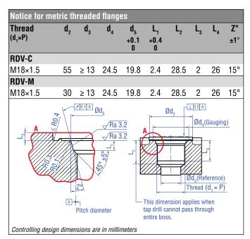
Fig. 42: Notice for metric threaded flange M18×1.5-6g based on DIN ISO 6149-1
