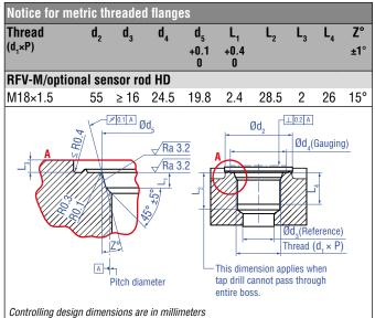
Fig. 36: Notice for metric threaded flange M18×1.5-6g based on DIN ISO 6149-1
