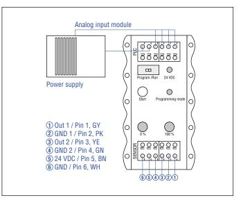
Fig. 105: Connect cabinet programmer
