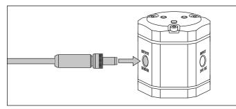
Fig. 84: Connection of adapter cable to TempoLink® smart assistant
