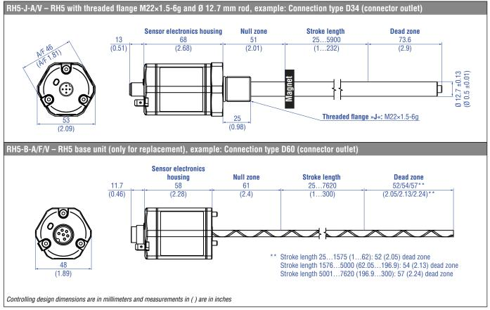
Fig. 7: Temposonics® RH5 with ring magnet, part 2
