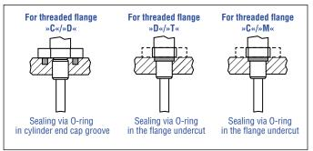
Fig. 41: Possibilities of sealing
