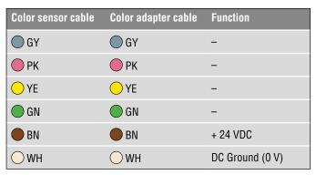
Fig. 86: Connection of adapter cable to sensor cable
