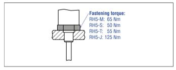
Fig. 8: Mounting example of threaded flange
