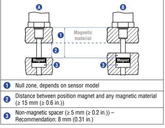
Fig. 51: Installation with magnetic material
