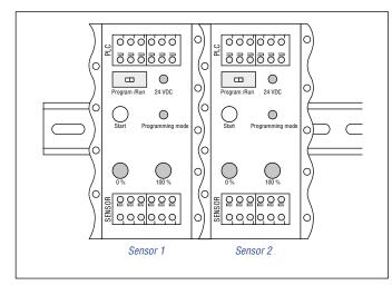
Fig. 104: Installation of cabinet programmer on a 35 mm standard rail
