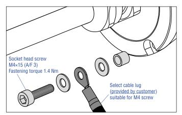
Fig. 73: Installation example for grounding of RM5 sensor
