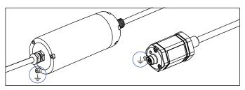
Fig. 72: Grounding via ground lug on the example of an RM5 sensor (left)/RH5 sensor (right)
