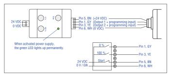
Fig. 103: Connect hand programmer
