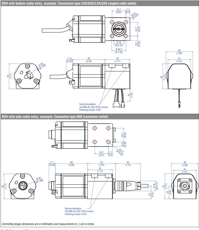
Fig. 37: Temposonics® RDV sensor electronics housing, part 1
