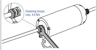
Fig. 71: Replacement of the base unit on model RM5, part 4
