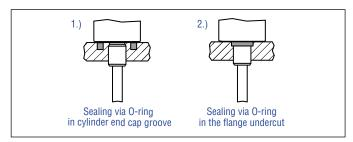
Fig. 15: Possibilities of sealing
