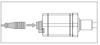
Fig. 85: Connection of adapter cable to R-Series V sensor with connector outlet
