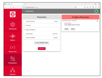
Fig. 97: Download a cek file with the settings of the sensor
