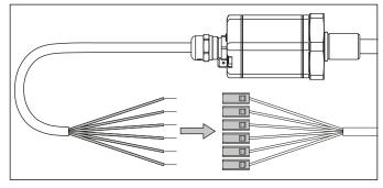
Fig. 87: Connection of adapter cable to R-Series V sensor with cable outlet
