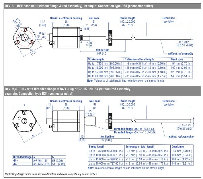
Fig. 28: Temposonics® RFV with ring magnet, part 1
