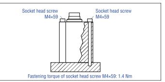
Fig. 32: Mounting with socket head screws M4×59
