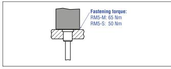
Fig. 13: Mounting example of threaded flange
