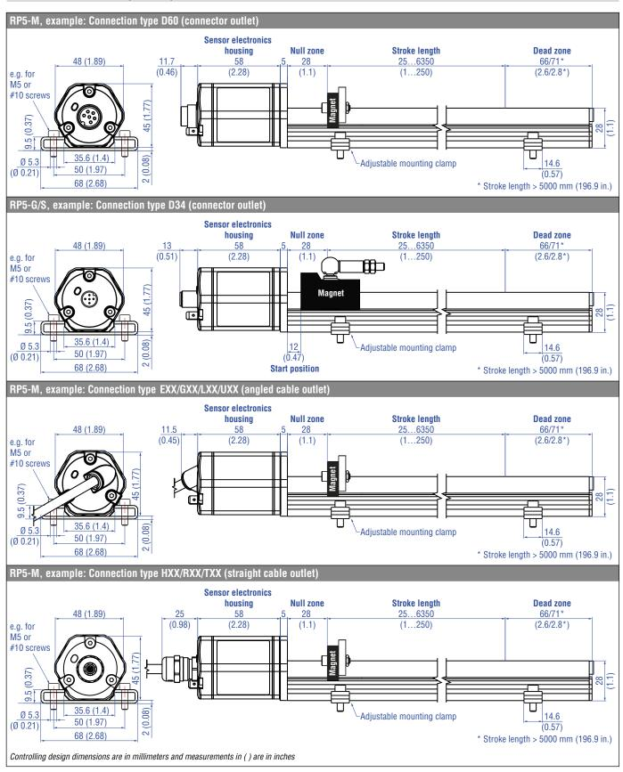
Fig. 3: Temposonics® RP5 with U-magnet/magnet slider
