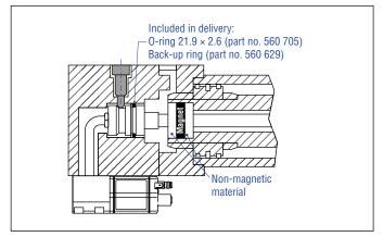
Fig. 45: Mounting example of pressure fit flange  ${}^{\rm >}S{}^{\rm <}$  and sensor electronics with bottom cable entry
