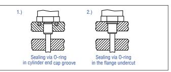
Fig. 25: Possibilities of sealing
