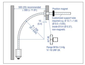
Fig. 31: Clearances for installation and handling
