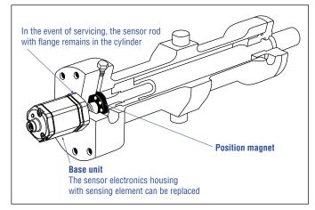
Fig. 9: Sensor in cylinder
