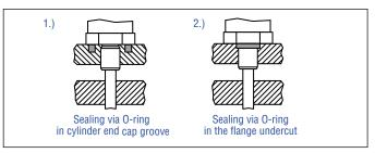
Fig. 35: Possibilities of sealing
