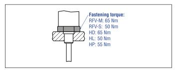
Fig. 33: Mounting example of threaded flange
