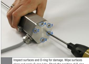
clean and apply O-ring lube. Check the position of O-ring between upper lid and connection adapter.
