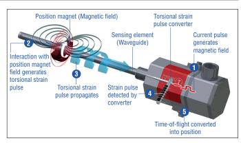
Fig. 3: Time-of-flight based magnetostrictive position sensing principle
