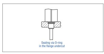
Fig. 11: Possibility of sealing for threaded flange with raised-face
