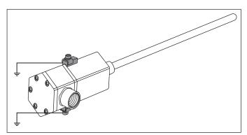
Fig. 21: Grounding via ground lug
