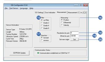
Fig. 33: Temposonics SSI-Configurator, Measurement
