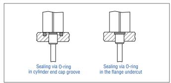
Fig. 12: Possibilities of sealing for threaded flange with flat-face
