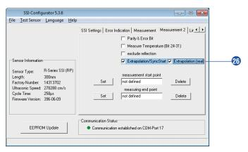
Fig. 35: Temposonics SSI-Configurator, Measurement 2, choose "synchronous mode 3"
