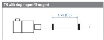
Fig. 19: Minimum distance between magnets for differentiation measurement
