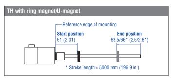
Fig. 18: Start and end positions of magnets
