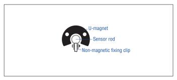
Fig. 17: Example of sensor support (part no. 561 481)
