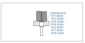
Fig. 9: Mounting example of threaded flange
