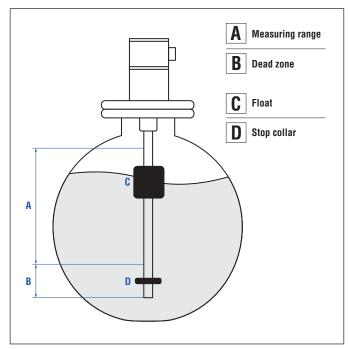
Fig. 20: Liquid level measurement
