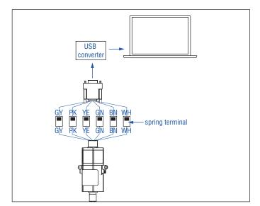
Fig. 29: Connect PC programmer
