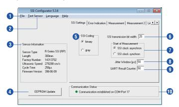
Fig. 30: Temposonics SSI-Configurator, SSI Settings
