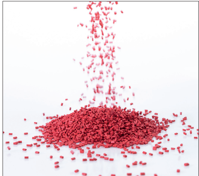
Fig. 2: Plastic granulate for injection molding or extrusion
