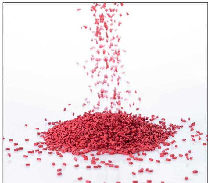
Fig. 2: Plastic granulate for injection molding or extrusion
