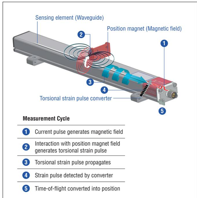
Fig. 1: Time-of-flight based magnetostrictive position sensing principle
