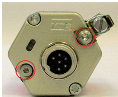
Fig. 2: Fasten screws with 1,3 Nm
