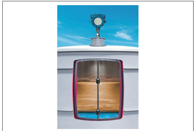
Fig. 2: Example of product and interface level measurement
