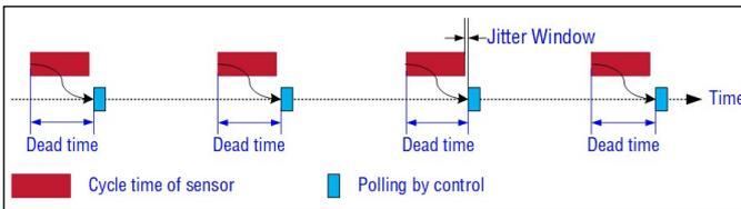
Fig. 4: Schematic representation of synchronous mode 1 for R-Series V SSI
