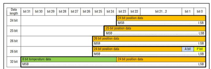
Fig. 2: Structure of the SSI transmission telegram for the R-Series V SSI with different data length with alarm bit (A bit) and parity bit (P bit)
