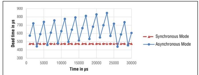
Fig. 5: Dead time in asynchronous and synchronous mode in the course of time
