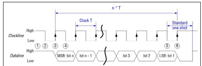
Fig. 1: Timing diagram of an SSI data transmission with a data length of  $n$  bits
