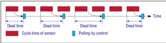
Fig. 3: Schematic representation of asynchronous mode for R-Series V SSI
