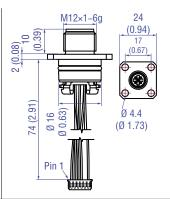
5 pin mating connector cable M12 Part no. 254 560
