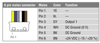
Fig. 13: Connector wiring with extension cable 254 642-x
