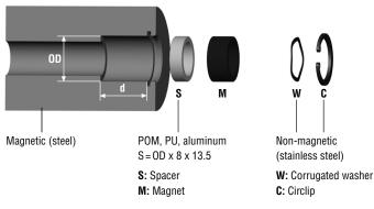
Fig. 6: "Position magnet in piston" installation example
