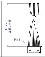
Mating connector cable pigtail Part no. 254 266
