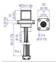
5 pin mating connector cable M12 Part no. 254 256
