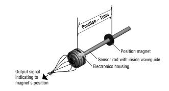
Fig. 1: Principle of operation:
