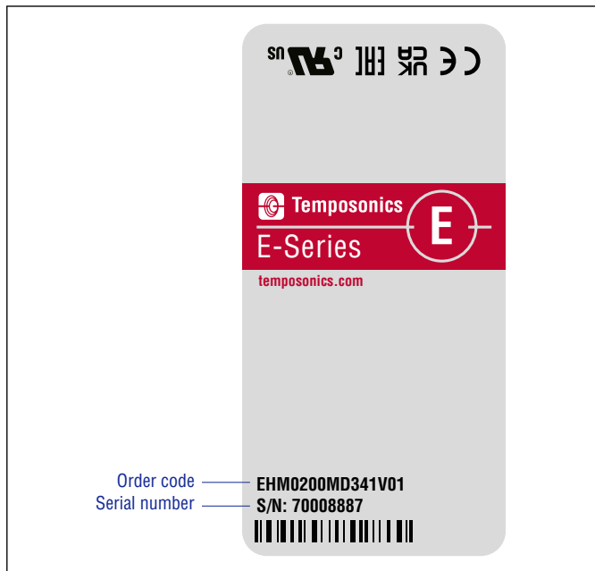
Fig. 1: Example of nameplate of E-Series EH sensor with Analog output
