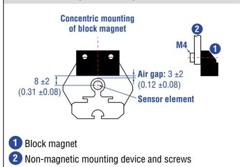
Magnet mounting with magnetic material
