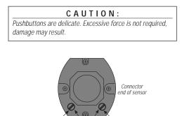
Remove screws to access zero and span pushbuttons.
