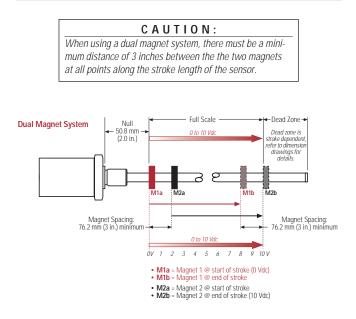
In the following procedure, Magnet #1 is the magnet closest to the head of the sensor.
