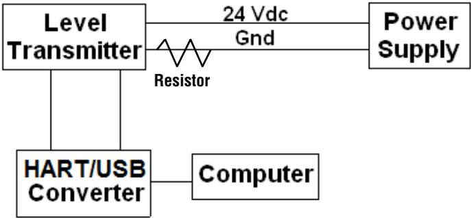
Fig. 3: Example setup
